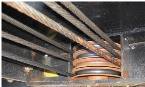
Rust on sheave stack and ropes
